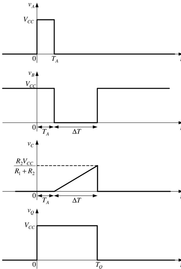
$$T_Q = T_A + \Delta T = T_A + \frac{R_2 V_{CC} C_1}{(R_1 + R_2) I_0}$$
