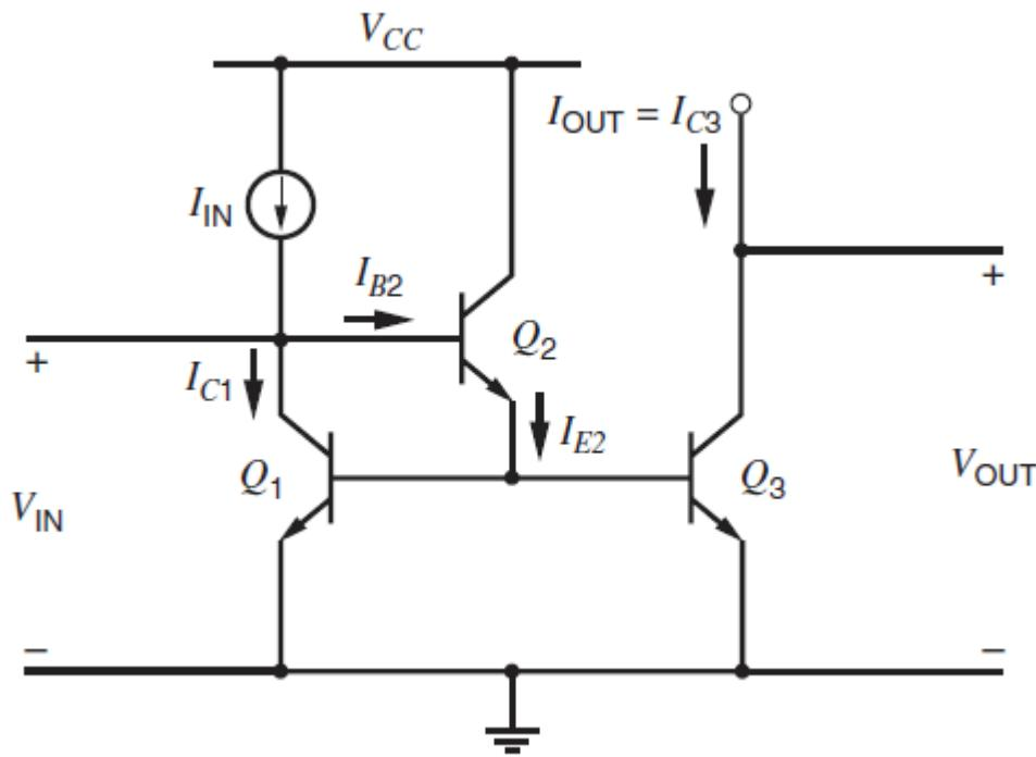
$$V_{IN} = V_{BE1(on)} + V_{BE2(on)}$$
