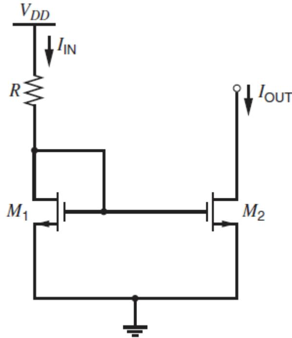
$$I_{IN} = \frac{V_{DD} - V_{GS1}}{R}$$
