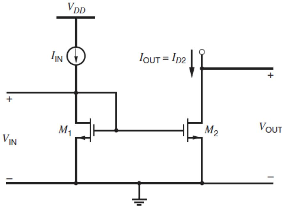
$$V_{GS1} = V_{GS2}$$
