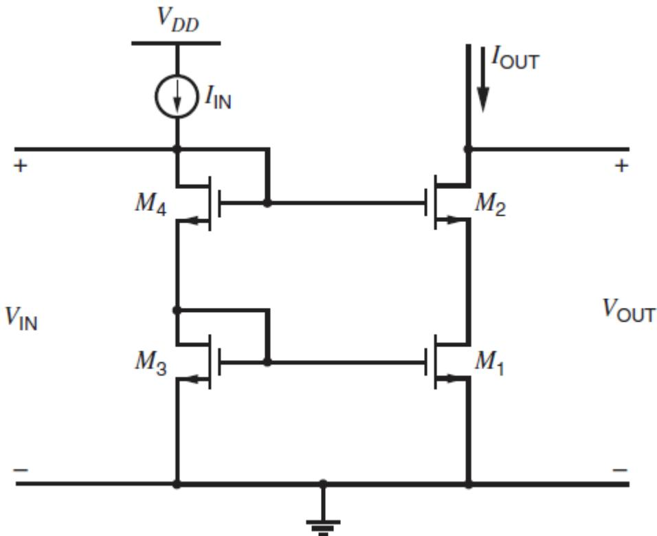
$$V_{IN} = V_{GS3} + V_{GS4}$$
