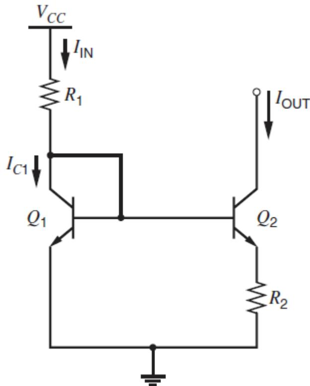
$$V_{BE1} - V_{BE2} - \frac{\beta_F + 1}{\beta_F} I_{\text{OUT}} R_2 = 0$$
