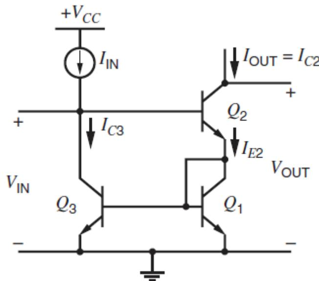
$$V_{IN} = V_{CE3} = V_{BE1} + V_{BE2} = 2V_{BE(on)}$$
