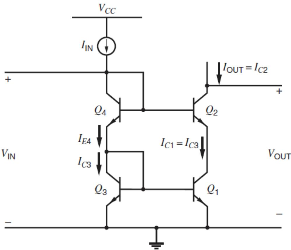
$$V_{IN} = V_{BE3} + V_{BE4} = 2V_{BE(on)}$$
