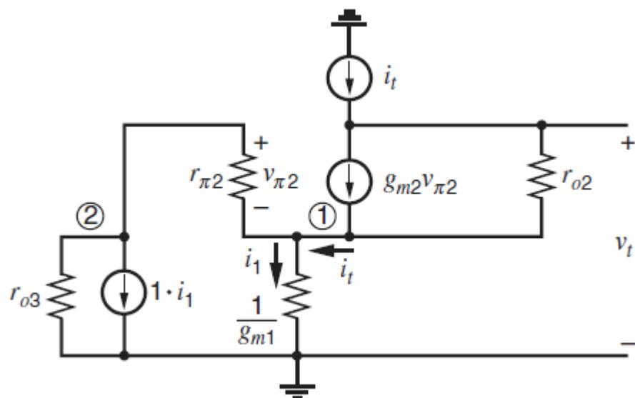
$$i_1 = \frac{i_t}{1 + \left( \frac{1}{1 + \frac{g_m1 r_{o3}}{1 + \frac{r_{\pi2}}{r_{o3}}}} \right)}$$
