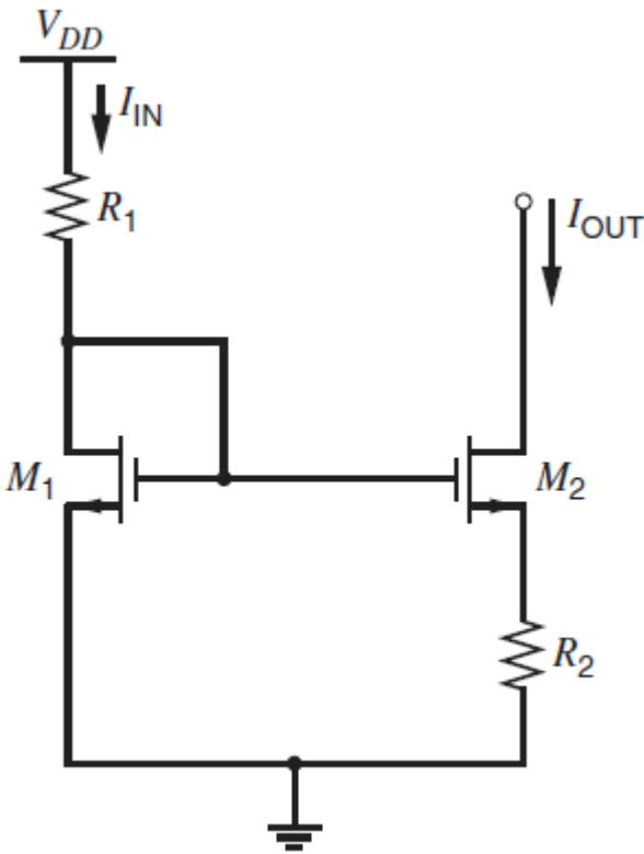
$$I_{D1} = I_{IN} = \frac{V_{DD} - V_{GS1}}{R}$$
