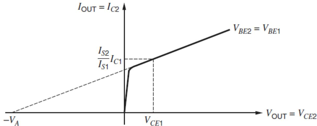
$$I_{\text{OUT}} = \frac{I_{S2}}{I_{S1}} I_{C1} \left( 1 + \frac{V_{CE2} - V_{CE1}}{V_A} \right) = \frac{\frac{I_{S2}}{I_{S1}} I_{\text{IN}} \left( 1 + \frac{V_{CE2} - V_{CE1}}{V_A} \right)}{1 + \frac{1 + (I_{S2}/I_{S1})}{\beta_F}}$$
