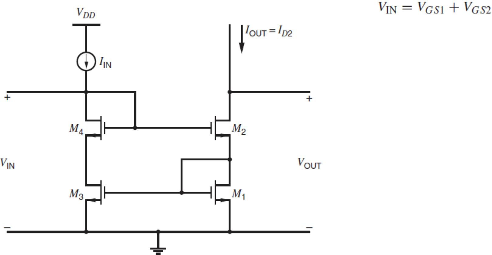
$$R_o = \frac{1}{g_{m1}} + r_{o2} + g_{m2}r_{o2} \left( 1 + \frac{1}{g_{m1}r_{o3}} \right) r_{o3} \simeq (1 + g_{m2}r_{o3})r_{o2}$$
