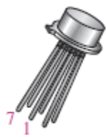
(a) Dual metal can. Emitters are closest to tab.
