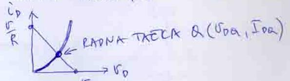
ANALITIČKI: RADI SE ITERATIVNO:  $i_D = I_S (e^{\frac{V_D}{V_T}} - 1) \Rightarrow V_D \approx \ln\left(\frac{i_D}{I_S}\right) \cdot V_T$
