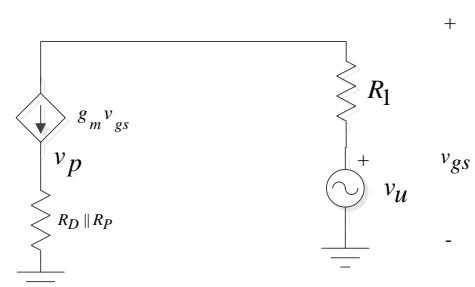
$$R_u = \frac{v_u}{g_m v_{gs}} = R_l + \frac{1}{g_m}$$
