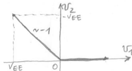
$$\begin{aligned} b) v_1 > 0 &\Rightarrow D_1 \text{ ON}, D_2 \text{ OFF} \Rightarrow v_2 = v_1 \\ \text{KADA } A_1 \text{ UVE} &\text{ U NEGATIVNO 2ASICE/IE} \\ \text{TADA JE } v_2 = 2v_{A2}^+ - (V_{EE} + V_0), v_{A2}^+ = \frac{v_1 + (V_{EE} + V_0)}{2} \\ &\Rightarrow v_2 = v_1 \\ v_1 < 0 &\Rightarrow D_2 \text{ ON}, D_1 \text{ OFF} \Rightarrow v_2 = -v_1 \\ v_1 = 0 &\Rightarrow v_2 = 0 \end{aligned}$$
