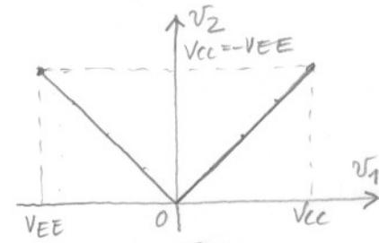
$$\begin{aligned} c) v_1 > 0 &\Rightarrow D_1 \text{ ON}, D_2 \text{ OFF} \Rightarrow v_2 = v_1 \\ v_1 < 0 &\Rightarrow D_2 \text{ ON}, D_1 \text{ OFF} \Rightarrow v_2 = 0 \\ v_1 = 0 &\Rightarrow v_2 = 0 \end{aligned}$$
