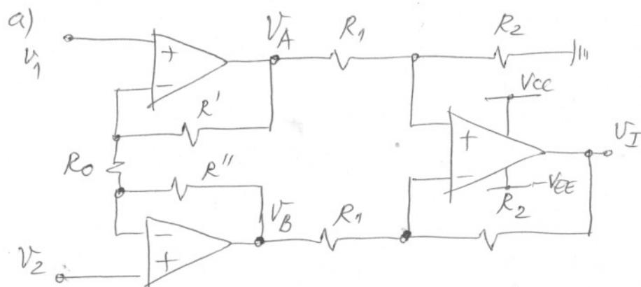
b)  $A_1 = 1 + \frac{R' + R''}{R_0} = 10$        $\frac{R' + R''}{R_0} = 9$        $R' = R''$        $\frac{R'}{R_0} = 4,5$
