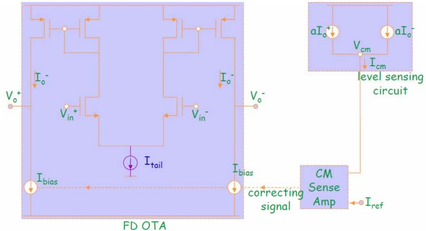
•Correcting signal can be voltage or current. Note that lo+, and lo- are equal to
