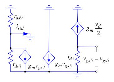
$$v_{gs5} = v_{gs7} = -r_{d1}g_m \frac{v_d}{2} \qquad r_{d1} = r_{ds1} || r_{ds3} || \frac{1}{g_m} \approx \frac{1}{g_m}$$
