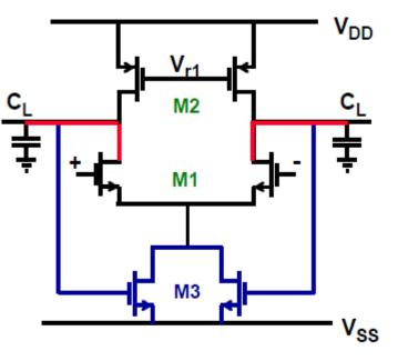
•It is clear that in the linear region, the transconductances are much smaller than in the saturation region. The common-mode  $\text{GBW}_{\text{CM}}$  is therefore smaller than the  $\text{GBW}_{\text{DM}}$ . This is a disadvantage!
