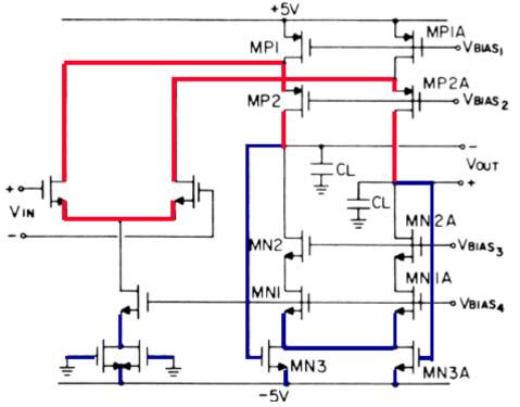
$\checkmark$  The main advantage of this first principle of CMFB is that no additional power is required. The main disadvantage is that this CMFB amplifier may not be sufficiently fast, depending on the application.
