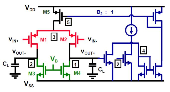
•Again, the output voltages are measured. The differential signals are cancelled out and the CMFB loop is closed by means of an amplifier.
