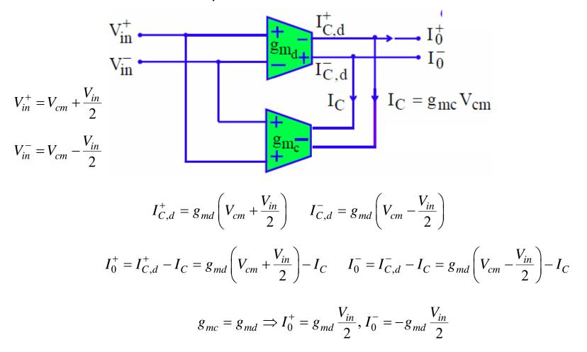
•Let us explore how a common-mode feedforward can be sensed and then applied. Consider a fully differential OTA with two current-mirrors
