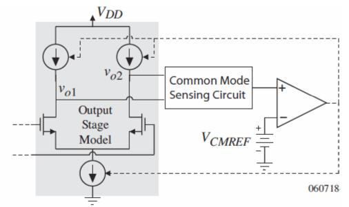
•Function of the common-mode feedback circuit:
