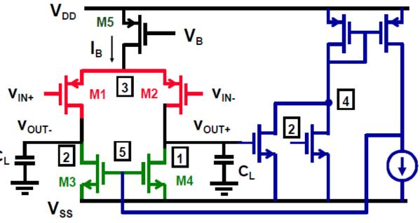
•Both output voltages are measured. Since we only want feedback on the common-mode signals, we have to cancel out the differential signals. This is done at node 4.
