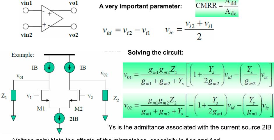
Fully-Differential Filters: Effects of current source impedance and mismatches
