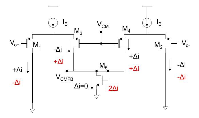
•Differential V<sub>o</sub>: V<sub>o+</sub> $\downarrow$  by  $\Delta$ V<sub>o</sub>, V<sub>o-</sub> $\uparrow$  by  $\Delta$ v<sub>o</sub> •Common mode V<sub>o</sub>: V<sub>o+</sub> $\uparrow$  by  $\Delta$ V<sub>o</sub>, V<sub>o-</sub> $\uparrow$  by  $\Delta$ v<sub>o</sub>
