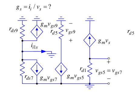
$$v_{s} = \frac{v_{1} + v_{2}}{2} \qquad v_{gs9} = -r_{d5}g_{m}v_{gs5}$$
