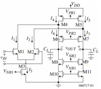
$$OCMR = V_{DD} + \left| V_{SS} \right| - V_{DSsatN} - V_{DSsatP}$$
