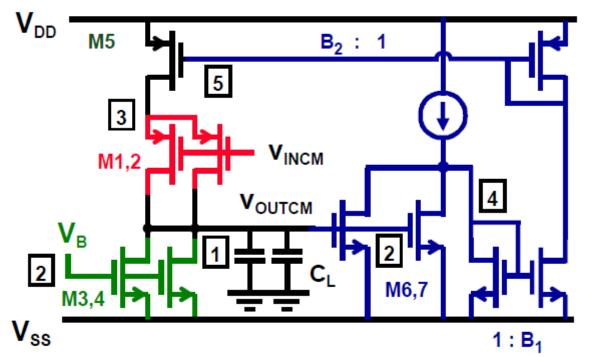
•Actually, the open-loop gain is  $B_1B_2g_{m5}R_{n1}$ . This gain is not so high but only a small amount of gain is needed.
