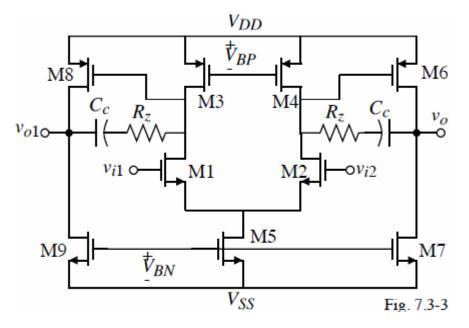
$$OCMR = V_{DD} + \left| V_{SS} \right| - V_{DSsatN} - V_{DSsatP}$$
