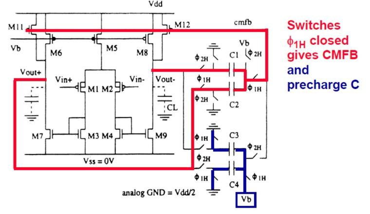
✓ In this slide, clock W1 is high, all the transistors, which are driven by this clock, are on. The other ones are off. Thick lines indicate which paths the signals can take. Clearly, the outputs are AC coupled by capacitors C1/C2. Their differential content is then cancelled out. Finally, this signal is then applied to the Gate of transistor M12 to close the feedback loop.
