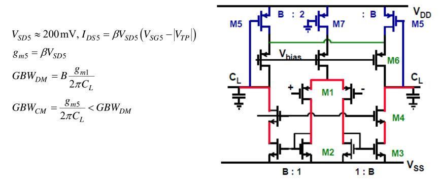
Two-Stage, Miller, Differential-In, Differential-Out Op Amp with Common-Mode Feedback
