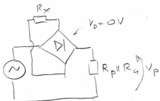
$$V_{Pm} = \frac{R_p \parallel R_4}{R_p \parallel R_4 + R_x} \cdot V_{sum} \quad - \text{vršne vrednosti}$$
