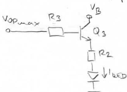
$$I_{LED\max} = \frac{V_{Pmax}}{R_2 + \frac{R_3}{\beta_3 + 1}} = \frac{10,26}{470 + \frac{18k}{121}} = 16,5 \text{ mA}$$
