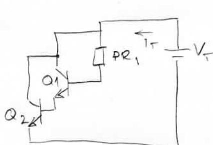
$$I_{B1} = \frac{V_T - V_{SE1} - V_{BE2}}{PR_1}$$
