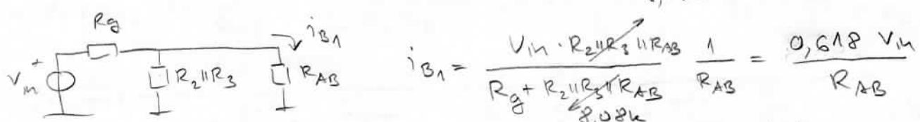
$$i_{B1} = \frac{V_m \cdot R_2 || R_3 || R_{AB}}{R_g + R_2 || R_3 || R_{AB}} \frac{1}{R_{AB}} = \frac{0,618 \text{ V}_m}{R_{AB}}$$
