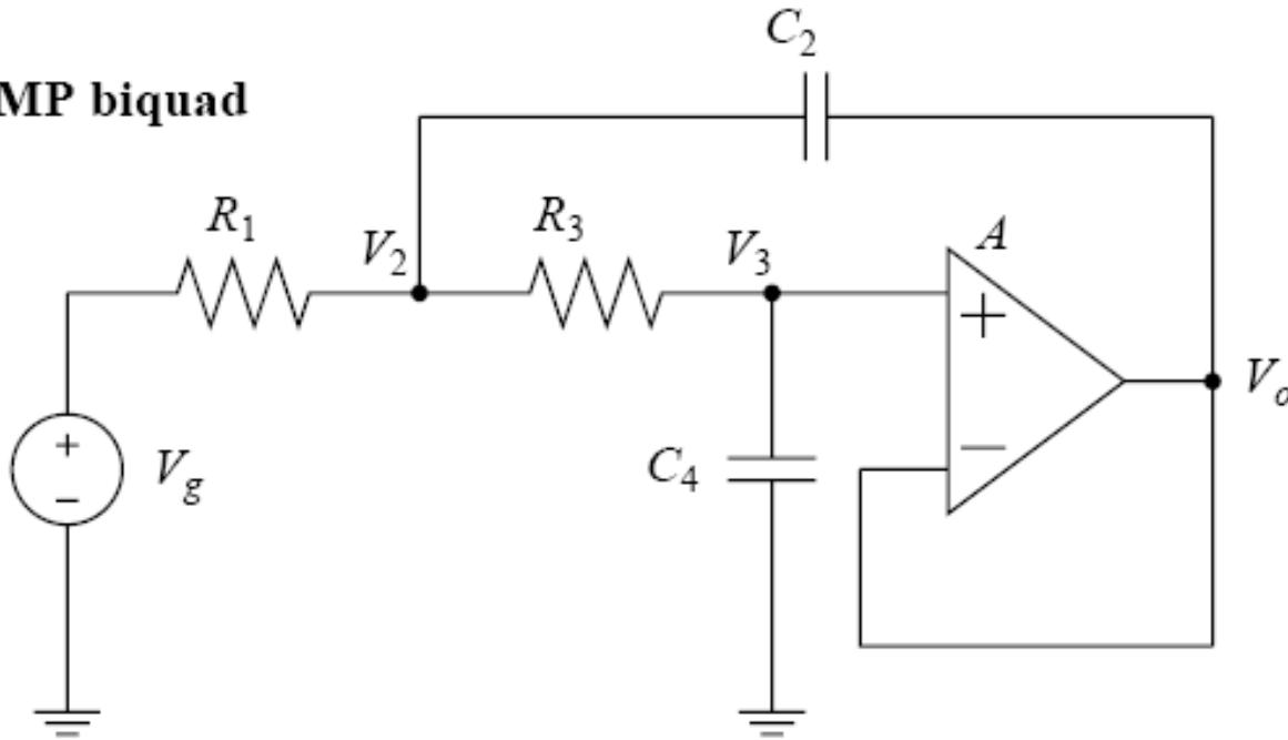
$$H(s) = \frac{\frac{1}{C_2 C_4 R_1 R_3}}{s^2 + \frac{R_1 + R_3}{C_2 R_1 R_3} s + \frac{1}{C_2 C_4 R_1 R_3}}$$
