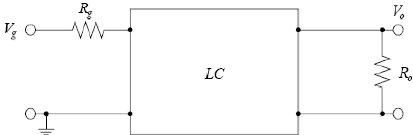
$$H(s) = \frac{V_o}{V_g} = \frac{R_o z_{21}}{R_g R_o + R_o z_{11} - z_{12} z_{21} + R_g z_{22} + z_{11} z_{22}}$$
