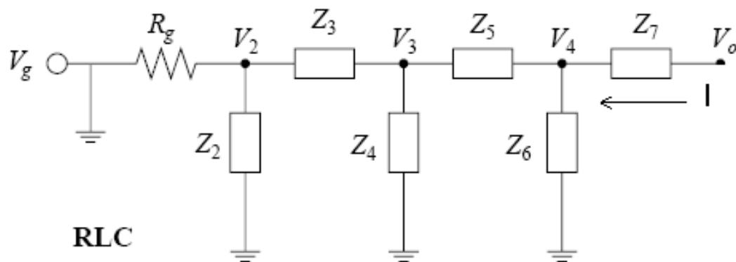
$$y_{22} = \frac{I_{Z_7}}{V_{Ro}}, \quad V_g = 0$$
